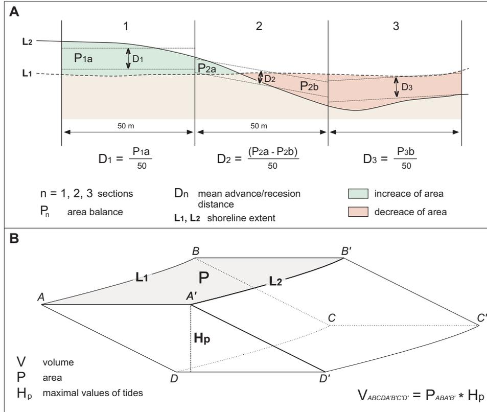
Fig. 6. Calculation schemes. **A.** The value of changes in shoreline range. **B.** The volume of material for tidal zone. See text for more explanation.
