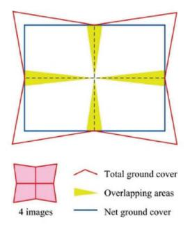
Fig. 1. Image stitching for imagery obtained by the Intergraph DMC-2001 sensor (Petrie G, 2008)
