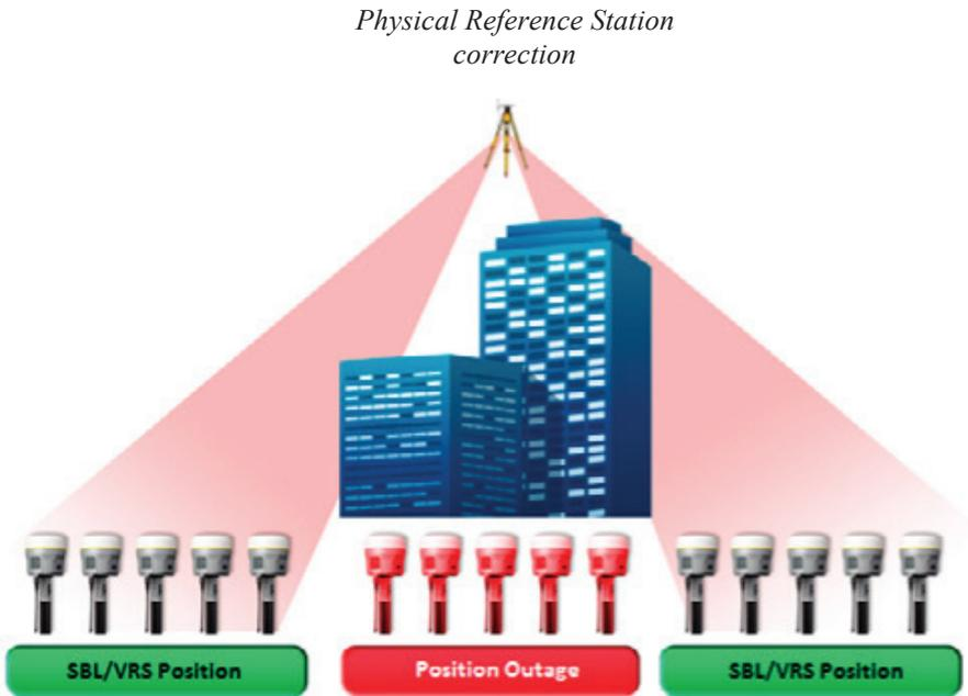
Fig. 2 RTK solution outage caused by a building obscuring the RTK radio signal (White Paper, 2012)
