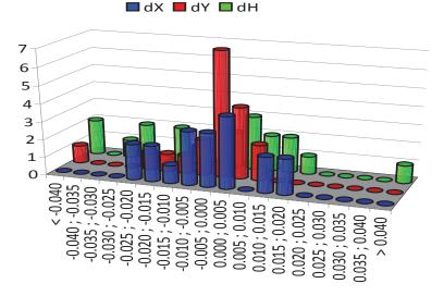
Fig. 7. Histogram of measured frequency for differences in coordinates between RTK-RTX methods
