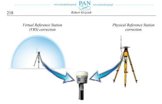
Fig. 1. Possible sources of corrections for most RTK systems: single physical reference station or VRS (White Paper, 2012)
