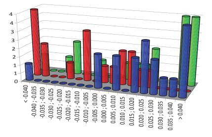
Fig. 8. Histogram of measured frequency for differences in coordinates between RTK-3rd class CAT. methods
