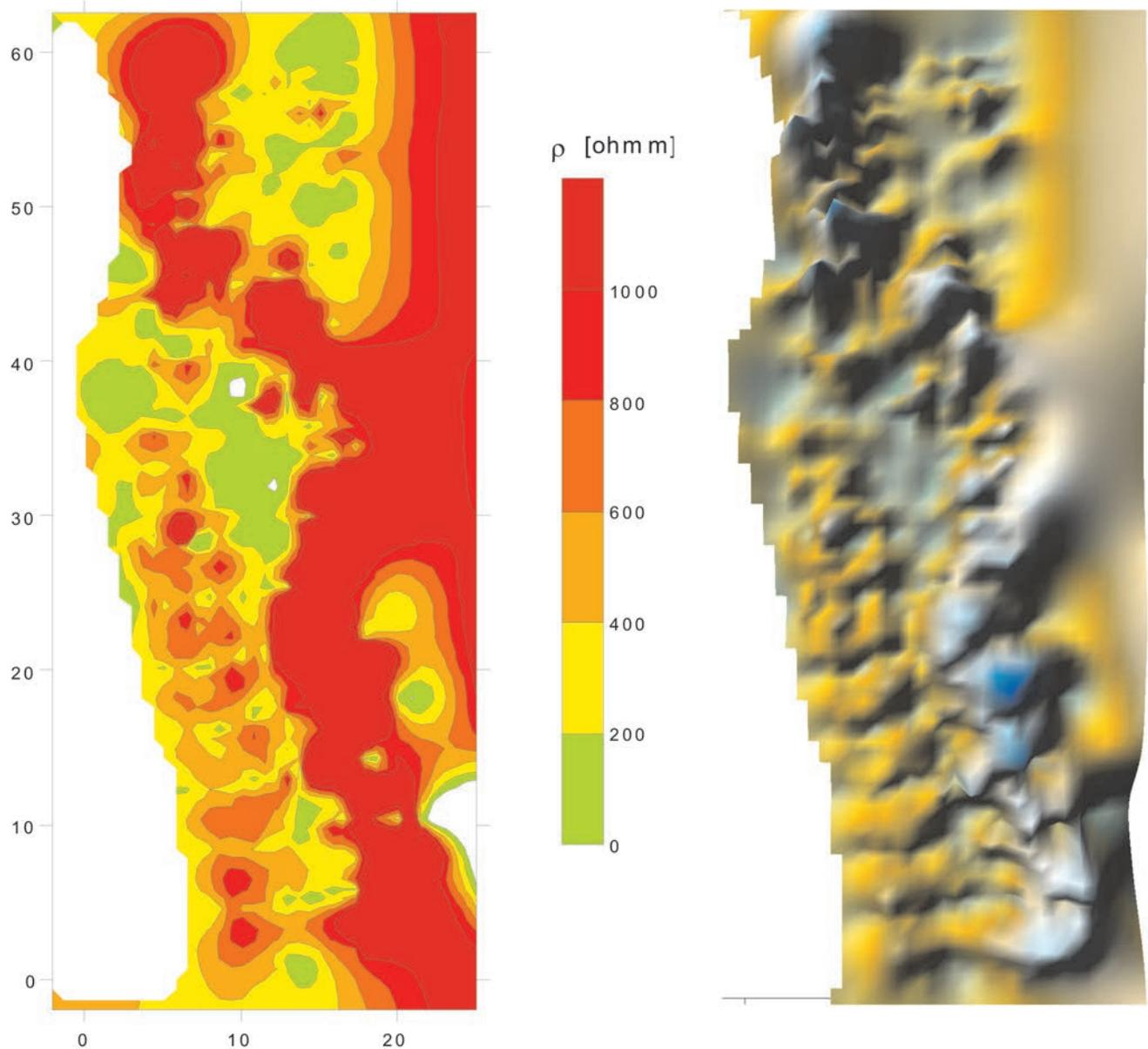
**Fig. 6.** Maps of apparent resistivity distribution in a rectangular array in 2D (left) and 3D (right) (modified from Mieszkowski and Porzeżyński, 2004).
