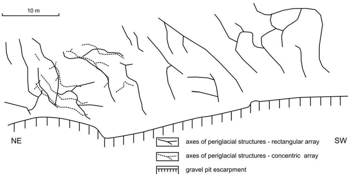
**Fig. 8.** Distribution of periglacial structures in the hinterland of the gravel pit escarpment at Wierzchuca Nagórna recognized by geological sounding (modified from Mieszkowski and Porzeżyński 2004)
