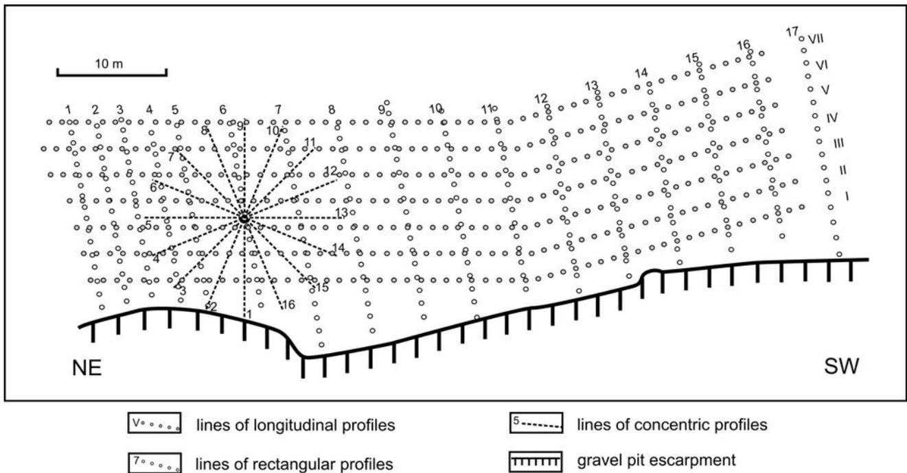
Fig. 4. Distribution of lines of geoelectrical sounding in a rectangular array and concentric array.
