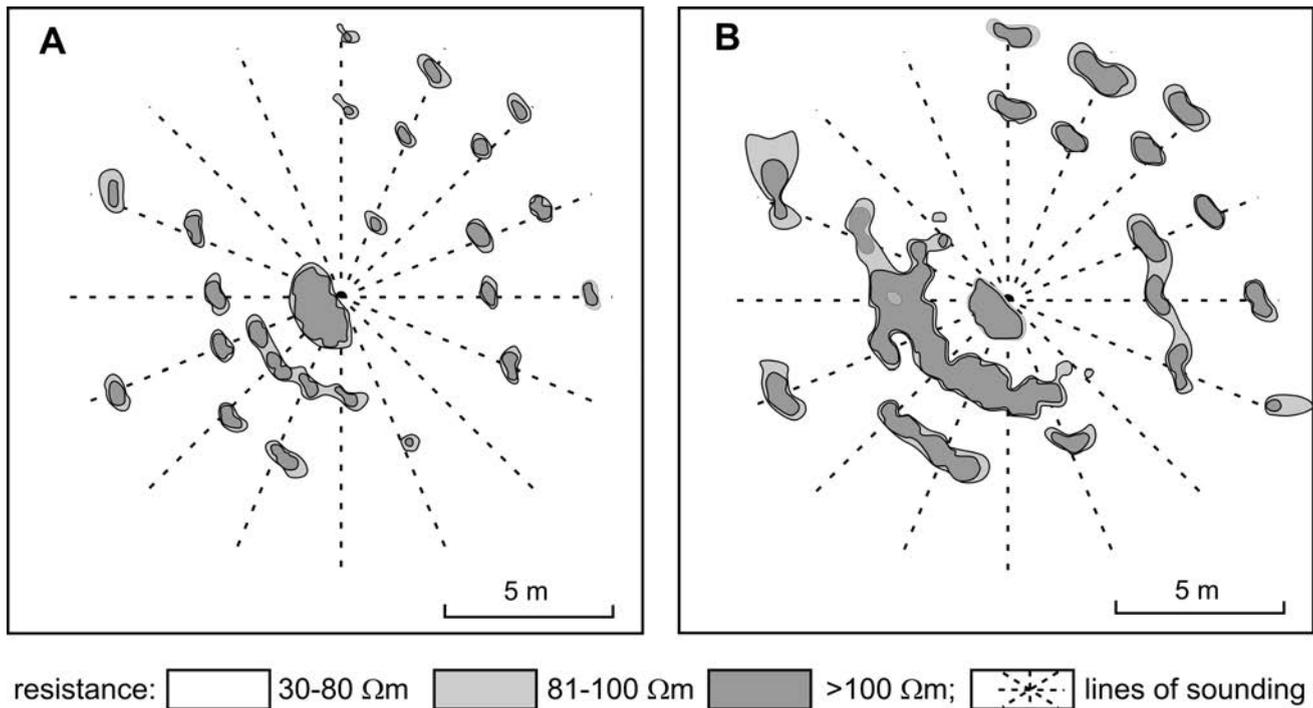
**Fig. 7.** Maps of apparent resistivity distribution in a concentric array (A), and 24 h after brine application (B) (modified from Mieszkowski and Porzeżyński, 2004).
