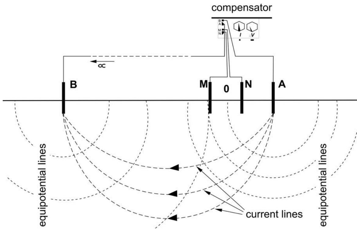
Fig. 1. Scheme of a non-symmetric measurement array.
