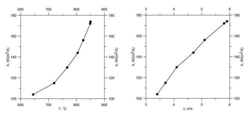
Figure 6. The heat transfer coefficient as a function of the flue gas temperature.
