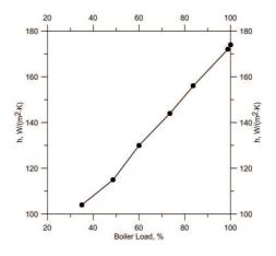
Figure 5. The heat transfer coefficient as a function of the boiler load.
