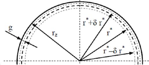
Figure 1: Figure of a cylinder cross-section with the outer radius ( $r_z$ ), the point of thermocouple installation ( $r^*, g$ ) and the accuracy of the thermocouple location ( $r^* + \delta r^*$ ,  $r^* - \delta r^*$ ).
