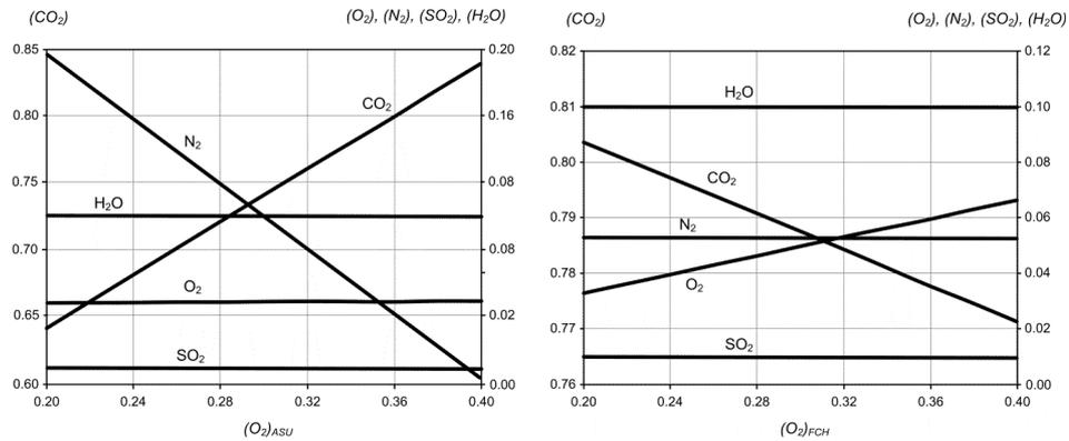
Figure 7: Composition of exhaust gas at the outlet from flue gas dryer as a function of oxygen content in oxidant: a) in FCH, b) in ASU.
