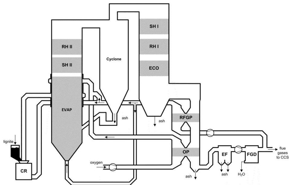
Figure 2: Profile of CFB boiler, other see Fig. 1.
