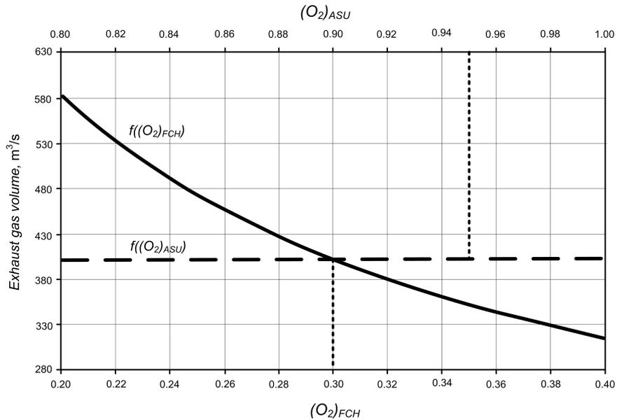
Figure 4: Exhaust gas volume as a function of oxygen content in oxidant.
