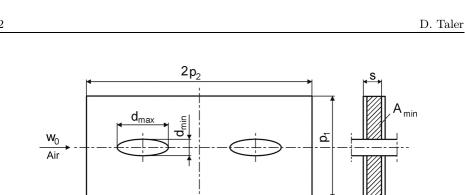
Figure 2. Cross section of two parallel tubes in the heat exchanger illustrating determination of the equivalent hydraulic diameter on the air side.
