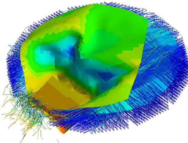
Fig. 10. Falling mass impact simulation for three platform artificial bottom with two additional cover plate layers – falling mass at rest
