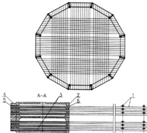
Fig. 1. Design solution of shaft artificial bottom
