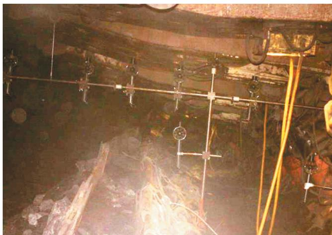
Fig. 2. The discussed section with visible sensors of the multi-point system for methane velocity and concentration measurements
