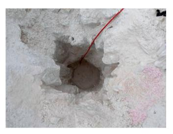
Fig. 3. Cracked hole collar and hardened plaster
