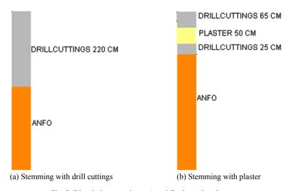
Fig. 2. Blast hole stemming at Asagi Caglayan basalt quarry
