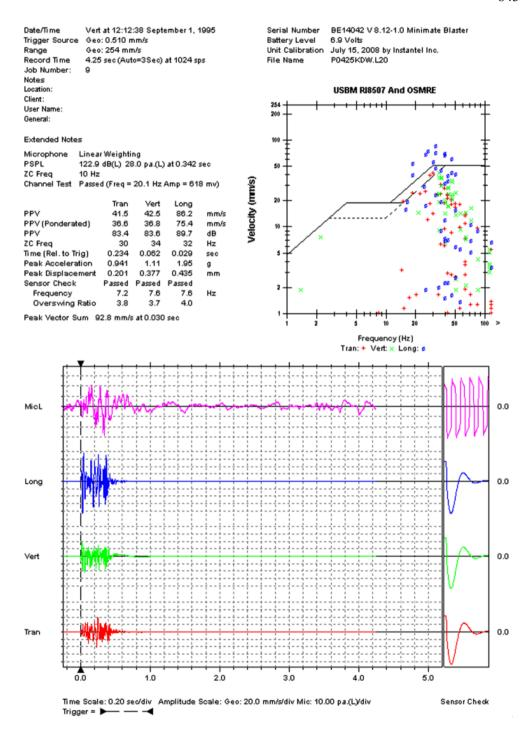
Fig. 6. Measured vibration and noise levels in the drill cuttings stemming test at Asagi Caglayan basalt quarry
