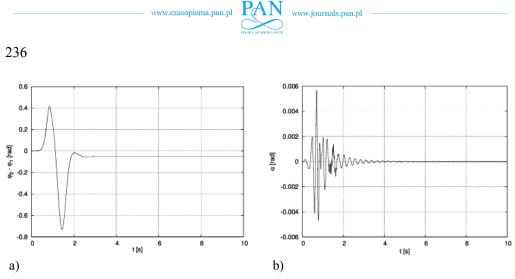
Fig. 8. Time-history of disphasing angle of vibrators  $\Delta \varphi$  (a) and angular coordinate  $\alpha$  (b) for suspension parameters presented in Table 1 – 4
