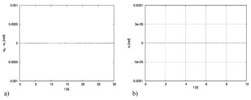
Fig. 7. Time-history of disphasing angle of vibrators  $\Delta \varphi$  (a) and angular coordinate  $\alpha$ (b) for suspension parameters presented in Table 1-3
