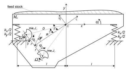
Fig. 2. Two-vibrator over-resonance vibratory machine in plane motion
