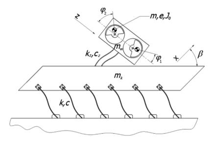
Fig. 1. Calculation model of over-resonance vibratory conveyor;
