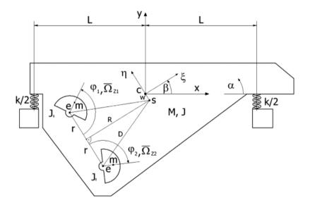
Fig. 3. Two-vibrator over-resonance vibratory machine calculation model.
