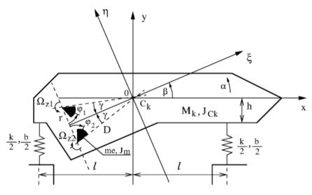
Fig. 4. Dynamic scheme of the vibratory machine.
