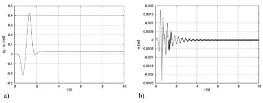
Fig. 6. Time-history of disphasing angle of vibrators  $\Delta \varphi$  (a) and angular coordinate  $\alpha$ (b) for suspension parameters presented in Table 1-2
