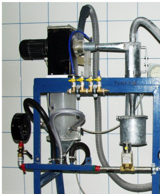
Fig. 4. Photograph of centrifugal flow classifier with fluidized bed
