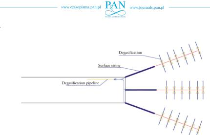
Fig. 3. Diagram of degasification method of prevention
