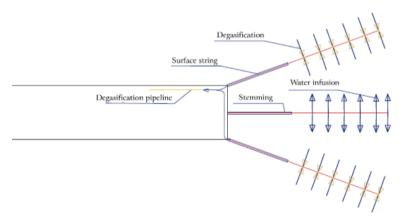
Fig. 5. Diagram of combined prevention method utilizing degasification and water infusion - 2<sup>nd</sup> variant
