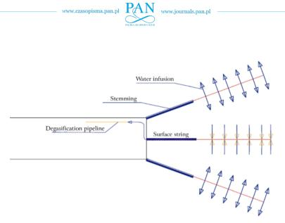
Fig. 4. Diagram of combined prevention method utilizing degasification and water infusion  $-1^{st}$  variant
