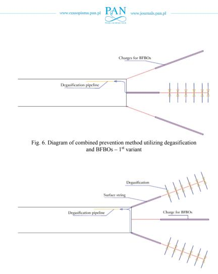
Fig. 7. Diagram of combined prevention method utilizing degasification and BFBOs  $-2^{nd}$  variant
