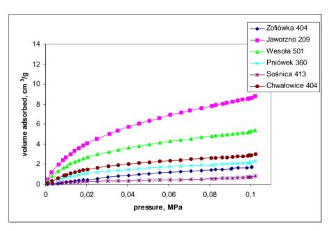
Fig. 3a. Isotherms of ethane sorption at 298 K on coals samples of different coals of 0,5-0,7 mm particle size
