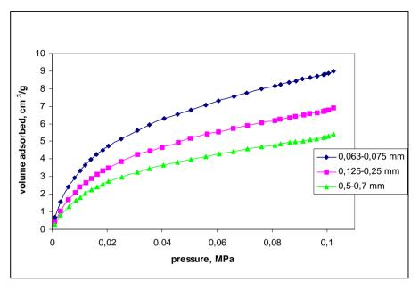
Fig. 4b. Isotherms of ethane sorption at 298 K on coal samples from Wesoła mine
