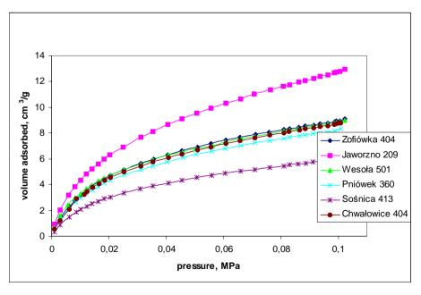
Fig. 3c. Isotherms of ethane sorption at 298 K on coals samples of different coals of 0,063-0,075 mm particle size
