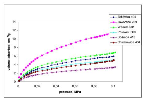
Fig. 3b. Isotherms of ethane sorption at 298 K on coals samples of different coals of 0,125-0,25 mm particle size
