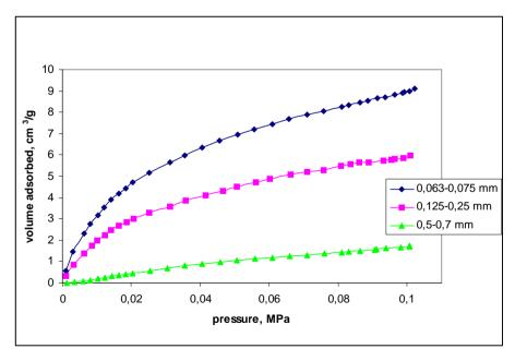
Fig. 5b. Isotherms of ethane sorption at 298 K on coal samples from Zofiówka mine
