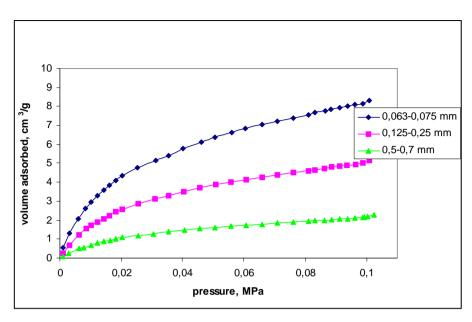
Fig. 5a. Isotherms of ethane sorption at 298 K on coal samples from Pniówek mine
