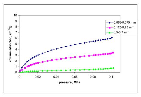
Fig. 5c. Isotherms of ethane sorption at 298 K on coal samples from Sośnica mine
