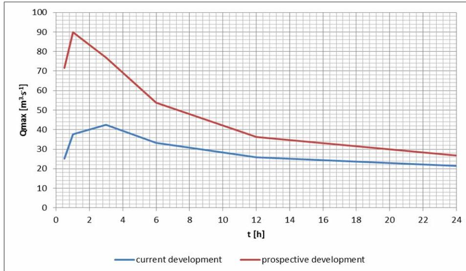
Fig. 2. The effect of watershed sealing on the size of  $Q_{\max 1\%}$  flows for different rainfall durations
