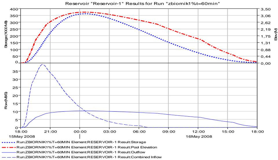
Fig. 4. Transformation of flood wave through a reservoir for the outflow of  $p = 1\%$  caused by precipitation with duration of 60 min
