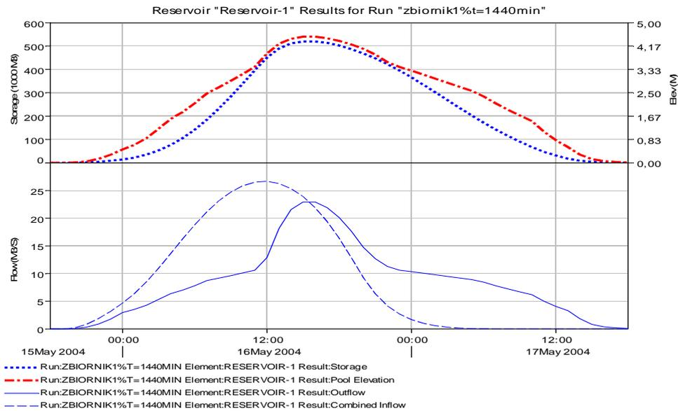
Fig. 5. Transformation of flood wave through a reservoir for the outflow of  $p = 1\%$  caused by precipitation with duration of 24 h
