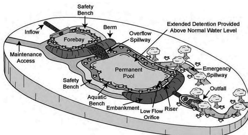
Fig. 3. Diagram of an extended retention flood detention reservoir [Wałęga 2010, after EPA 2007]
