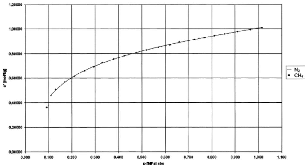
Fig. 1. Isotherm of adsorption of N<sub>2</sub> and CH<sub>4</sub> (Mg, Na – Clino) 298K
