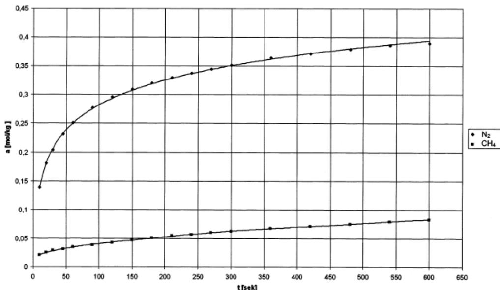
Fig. 2. Kinetics of adsorption of methane and nitrogen (Mg, Na – Clino) 298K
