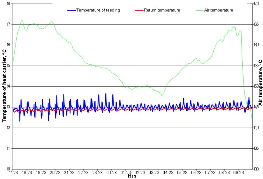
Fig. 7. Results of measurements of average temperature of rock mass for borehole P-1 (single U-tube) before TRT
