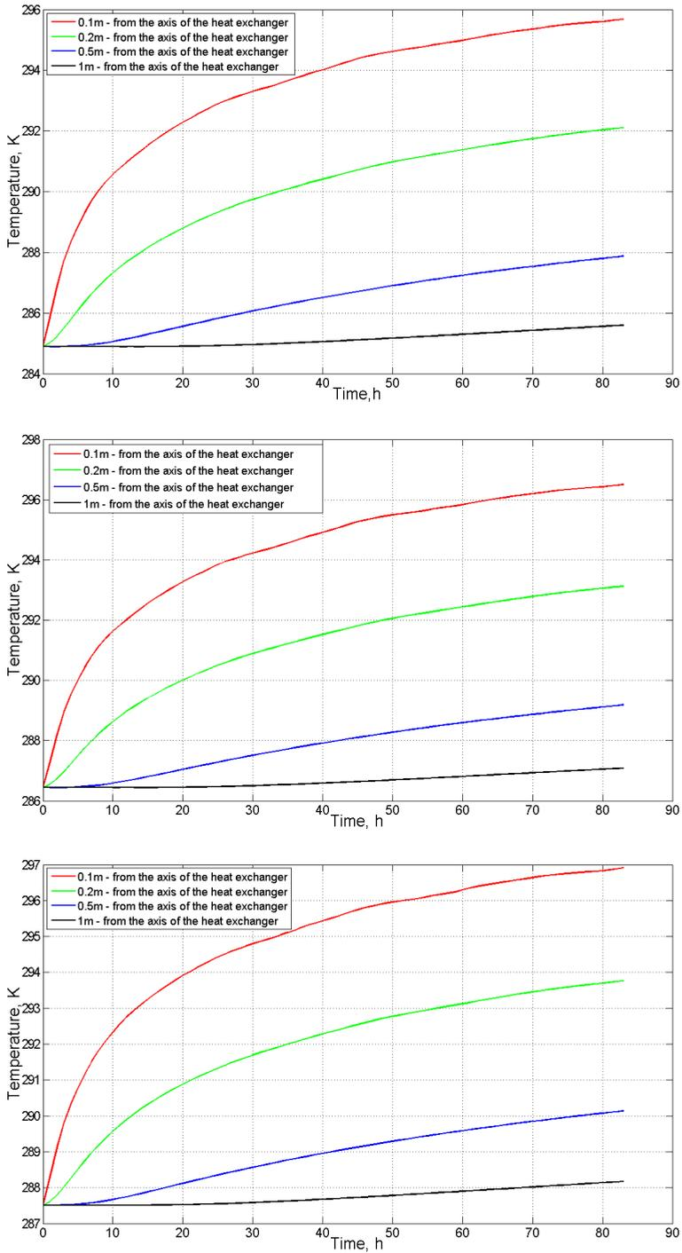
Fig. 12. Temperature changes in subsurface at a depth of 60 m, 120 m and 178 m, respectively
