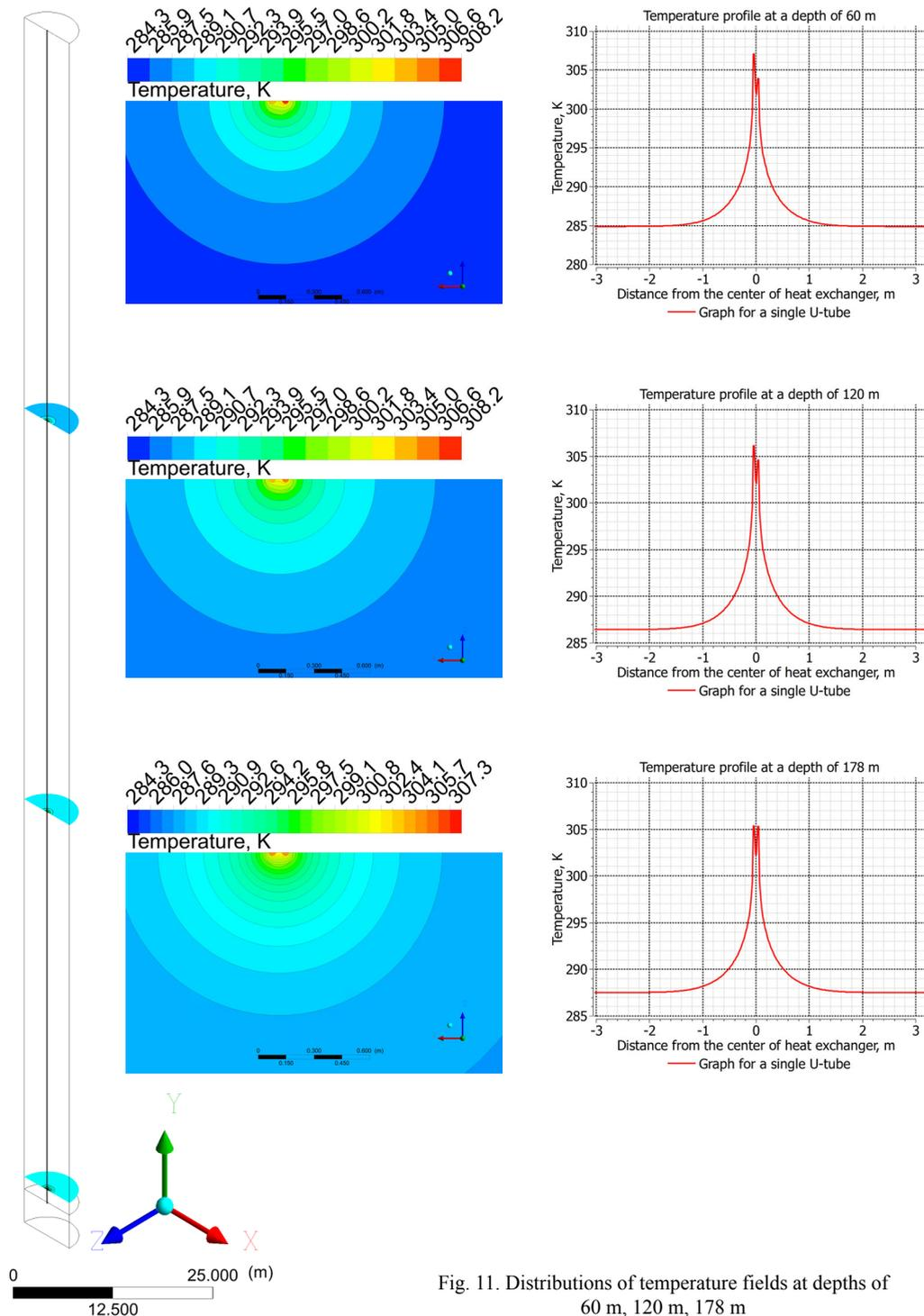
Fig. 11. Distributions of temperature fields at depths of 60 m, 120 m, 178 m
