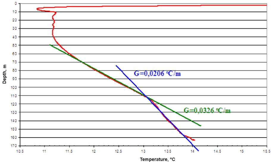
Fig. 6. Geothermal gradient in the hole P-2 (double u-tube) in terms of thermal stability
