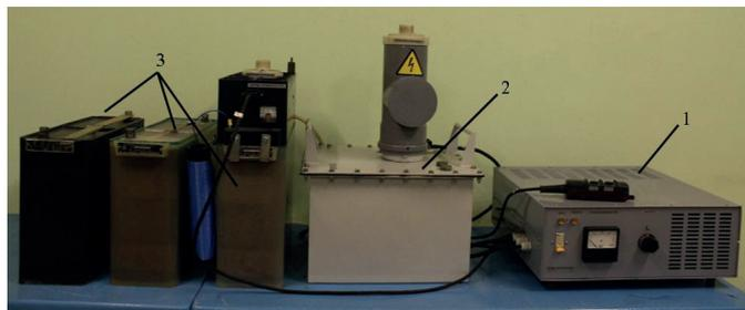
Fig. 1. An electric pulse plant. 1 – a control panel, 2 – a generator with a discharger, 3 – a protection unit with a capacitor
