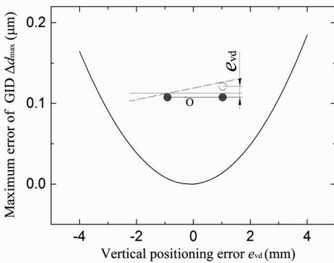
Fig. 15. The relation between  $\Delta d_{\max}$  and  $e_{vd}$ .
