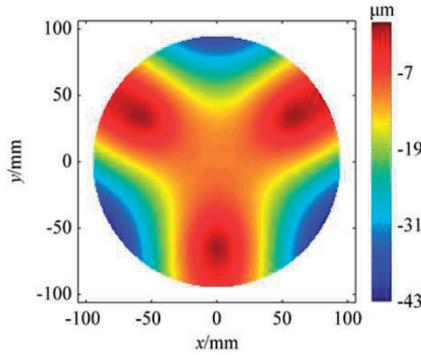
Fig. 4. The GID of a silicon wafer obtained using the FEM.
