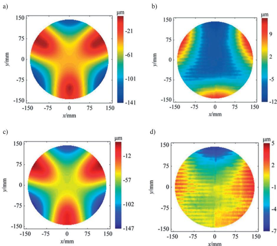
Fig. 9. a) The GID of the wafer obtained using the FEM without considering the effect of initial stress; b) difference of GIDs between those in Fig. 9a and Fig. 8b; c) the GID of the wafer obtained using the FEM considering the effect of initial stress; d) difference of GIDs between those in Fig. 9c and Fig. 8b.
