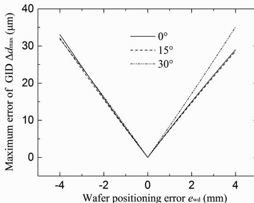
Fig. 19. The effect of  $e_{wd}$  in different directions on  $\Delta d_{max}$ .
