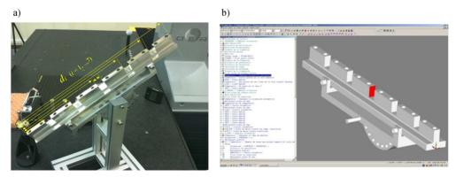
Fig. 1. a) The step gauge artefact with its seven standard lengths and the test setup for one of the 1st volume measuring orientation; b) a PCDMIS screen-capture for the off-line CAD programming.
