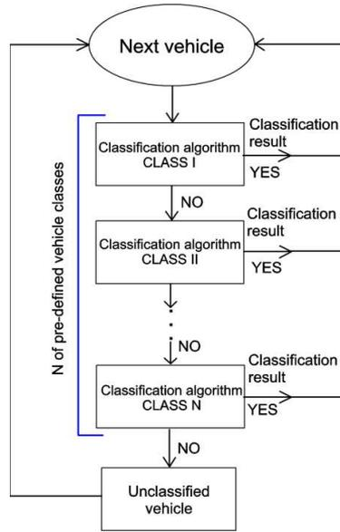
Fig. 8. Block diagram of the classification system.
