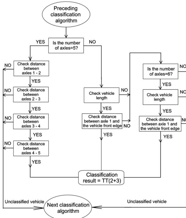
Fig. 9. Classification algorithm for TT(2+3) vehicle class.
