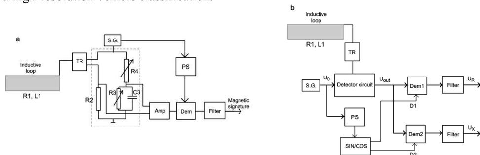
Fig. 1. Magnetic signature measuring systems: a) the bridge system, b) the system with separation of the detector impedance components. TR – transformer, S.G. – supplying generator, PS – phase shifter, Amp – amplifier, Filter – low-pass filter, Dem, Dem1, Dem2 – phase-sensitive demodulators, SIN/COS – signal generator,  $R1, L1$  – resistance and inductance of the loop.
