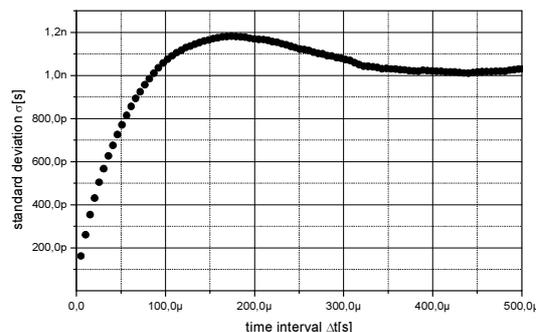
Fig. 7. Standard deviation as a function of time interval for reference clock EPSON F321G.
