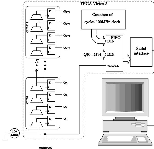
Fig. 1. Time interval measurement system based on a FPGA structure.
