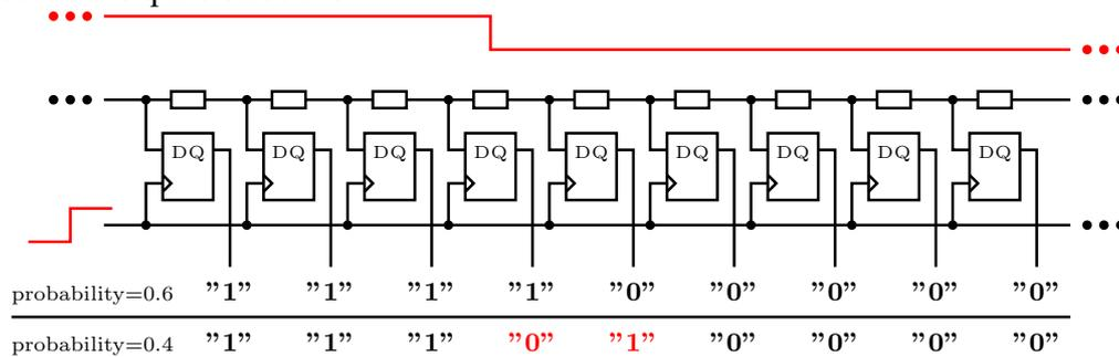
Fig. 6 Single element of TDL delay fluctuation.
