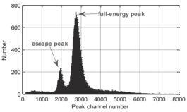
Fig. 18. Histogram of pulse distribution.
