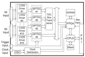
Fig. 3. Schematic of the time measurement module.
