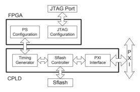
Fig. 9. Configuration of the FPGA.
