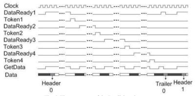
Fig. 6. Time sequence of the Parallel readout.
