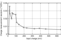
Fig. 17. Results of the charge measurement test.
