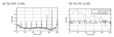
Fig. 11. Nonlinearity test results.
