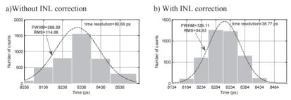
Fig. 12. Time resolution results with a -8 ns delay.
