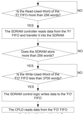
Fig. 8. State Machine of data buffer.
