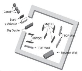
Fig. 1. Detector system of the CSR external target experiment.
