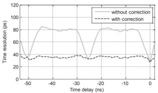
Fig. 13. Time resolution test results with different time delays.
