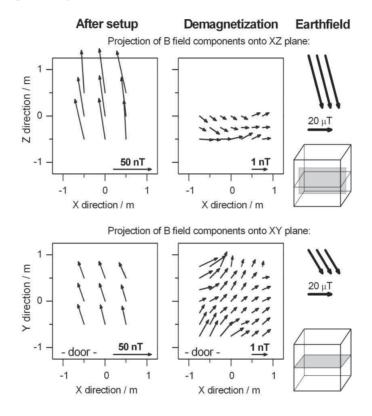
Fig. 5. Magnetic field map inside Zuse-MSR. Above:  $B_x$  and  $B_z$  components shown as projections onto the vertical plane. Below: projection of the  $B_x$  and  $B_y$  components onto a horizontal plane. Left: After installation of the MSR, using a fluxgate. Right: Result after degaussing using a SQUID system. Both measurements were performed at night during the subway break. Root points represent the measurement position. The origin corresponds to the center of the room.
