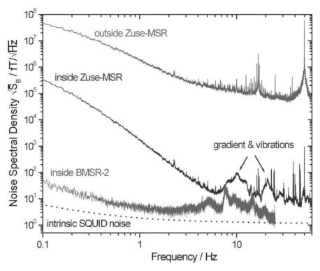
Fig. 7. Day time magnetic field noise inside BMSR-2 and Zuse-MSR measured with a SQUID system, compared to the surrounding urban field measured with a fluxgate. The behavior of the noise inside the Zuse-MSR is typical for a 2+1 layer MSR. The shielding factor at 0.1 Hz measured by the manufacturer is around 100 for the Zuse-MSR and 10<sup>6</sup> for BMSR-2.
