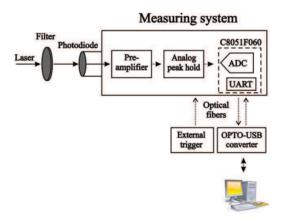
Fig. 1. Schematic drawing of the measuring system.
