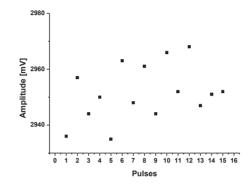
Fig. 4. Measured amplitude of the pulses, the average is 2946±12.3 mV.
