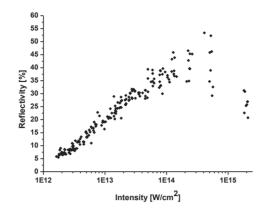
Fig. 8. Intensity dependence of the reflectivity for 620 fs KrF laser pulses.
