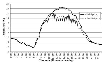
Fig. 6. The effect of daytime irrigation on the daily distribution of temperature on the day when the wind speed was lower than  $3 \text{ m} \cdot \text{s}^{-1}$ , and the relative humidity less than 50% at noon – in pear plantation – 23rd of April 2010
