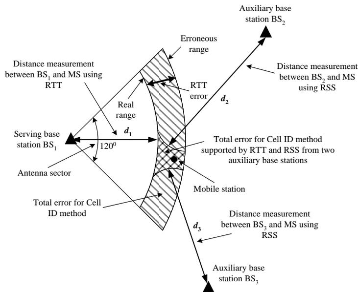
Fig. 1. Cell ID method supported by RSS.
