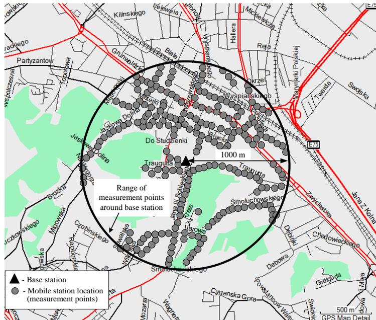
Fig. 2. View of a field test in the metropolitan area of Gdansk-Wrzeszcz<sup>6</sup>.
