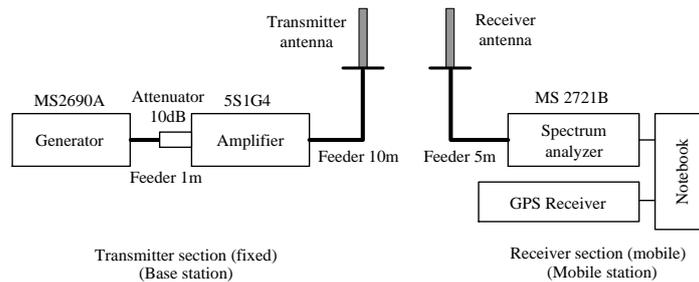
Fig. 3. Block diagram of measuring equipment set.
