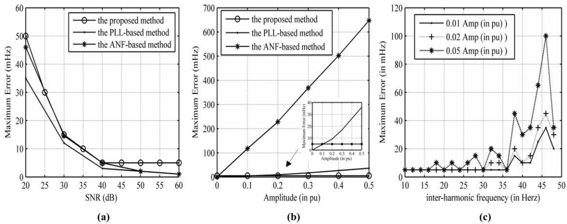
Fig. 2. Impact of (a) noise (b) harmonics (c) inter-harmonics on the estimated frequency.
