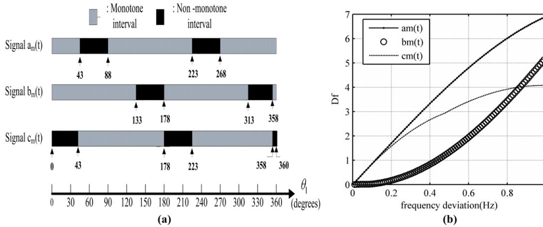
Fig. 1. (a) Monotone and non-monotone intervals for the modulating signal  $a_m(t)$ ,  $b_m(t)$  and  $c_m(t)$
