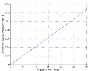
Fig. 9. Maximum absolute **reconstruction error** for test signal with white noise (*SNR*=90 dB) and matrix *F* **frequency deviation.**
