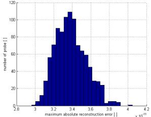
Fig. 13. Histograms of maximum absolute reconstruction error for a test signal with random phases (values from the uniform distribution in the interval [0°, 360°]). Left – signal with normal white noise (SNR=90 dB), right – signal without noise. Matrix F without error.
