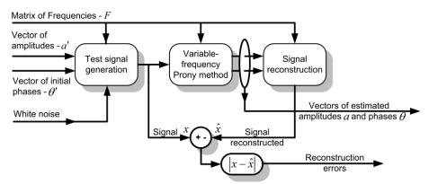
Fig. 2. Variable-frequency least squares Prony method - method for examination of parameter determination accuracy.
