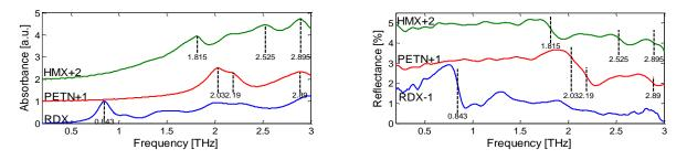
Fig. 9. Transmission and reflection spectra of RDX, HMX and PETN. Offsets (e.g.+1) for clarity.
