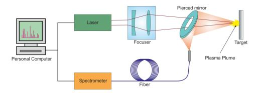
Fig. 4. LIBS experimental setup.
