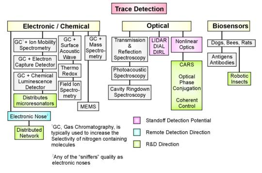
Fig. 3. Overview traces detection of explosives.
