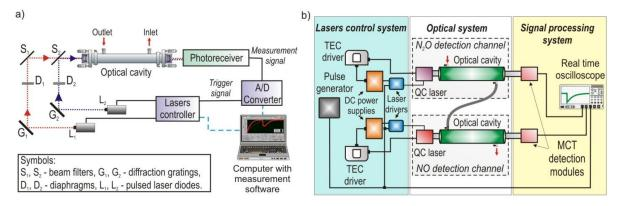
Fig. 11. Scheme of two-spectral CEAS sensor (a), simplified scheme of the experimental setup and example of the cavity output signals (b).
