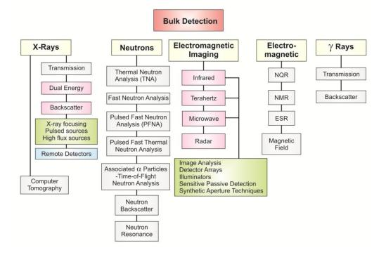
Fig. 2. Overview bulk detection of explosives.
