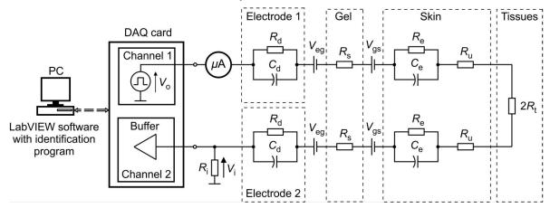
Fig. 4. System for identification of the skin-electrode interface.
