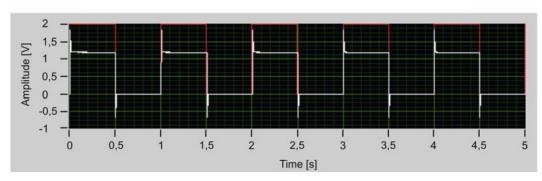
Fig. 7. Wave form of signal across the skin-electrode interface circuit in response to a square stimulus signal.
