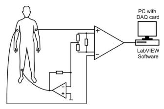
Fig. 8. System for signals registration at the skin-electrode interface output.
