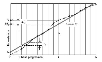
Fig. 1. Principle of jitter measurement through event timing.
