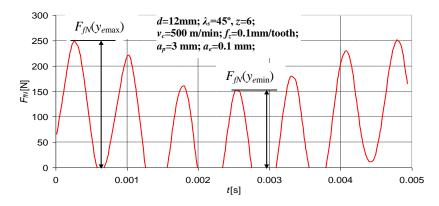
Fig. 2. The experimental time course of  $F_{fN}$  normal feed force component with the designation of instantaneous force corresponding to maximum  $F_{fN}(y_{emax})$  and minimum  $F_{fN}(y_{emin})$  cutter displacement envelope.
