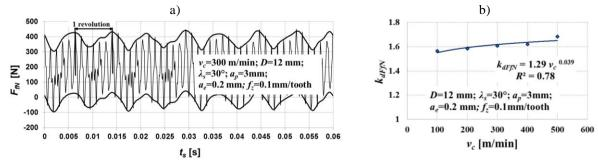
Fig. 5. a) time course for feed normal force component  $F_{fN}$  (thick black line denotes the envelope of  $F_{fN}$  force); b) dynamics coefficient  $k_{dFfN}$  in function of cutting speed  $v_c$ .
