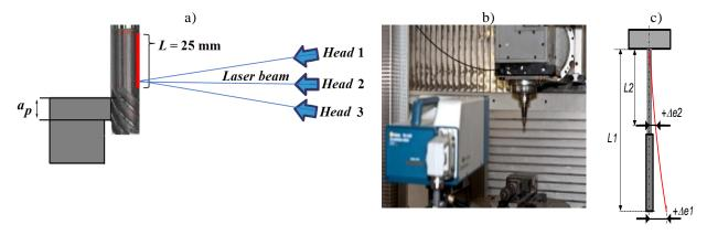
Fig. 4. Tool displacement measurement diagram: a) block scheme of 3D displacement measurement carried out on a scanning vibrometer; b) the view of laser head (no. 1) during the calibration process; c) the scheme of cutter displacement.
