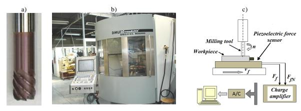
Fig. 3. Milling process experimental stand: a) the view of the employed tool; b) the view of DMG model DMU 60monoBLOCK milling center; c) block scheme of cutting force experimental apparatus.
