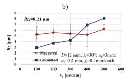
Fig. 9. a) surface roughness Ra in function of cutting speed  $v_c$ ; b) surface roughness Rz in function of cutting speed  $v_c$ .
