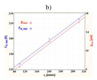
Fig. 8. a) maximum instantaneous displacement envelope  $y_{emax}$  per tool revolution in function of cutting speed  $v_c$ ; b) maximum instantaneous total displacement  $y_{max}$  per each tooth and feed normal force  $F_{fN\_RMS}$  in function of cutting speed  $v_c$ .
