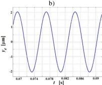
Fig. 7. a) the time course of measured total cutter displacement y (red line denotes the envelope of displacement  $y_e$ ) for  $v_c$ = 300 m/min; b) the time course of simulated envelope of cutter displacement  $y_e$  for  $v_c$ = 300 m/min.
