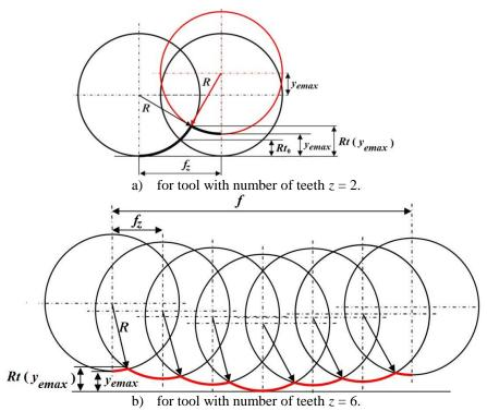
Fig. 1. Projection of the cutter into the work piece including cutter displacement, where: R – tool radius, f – feed per revolution,  $f_z$  – feed per tooth,  $y_{emax}$  – maximum value of cutter displacement envelope,  $Rt(y_{emax})$  – surface roughness height including cutter displacement,  $Rt_0$  – theoretical surface roughness.
