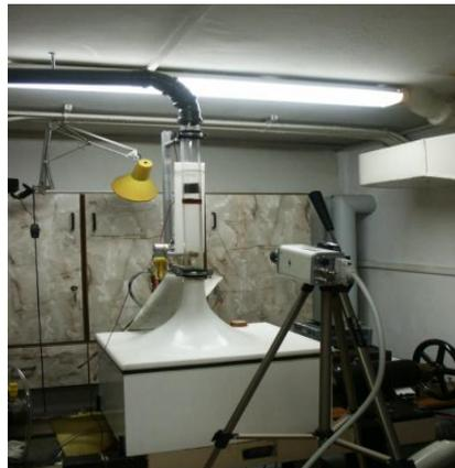
Fig. 6. Flow visualization measuring stand.
