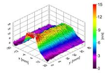
Fig. 11. Transverse velocity distribution for a circular cylinder with slit
