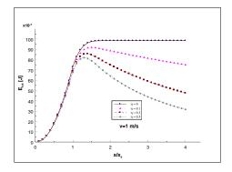
Fig. 4. Total rotation energy of the vortex as a function of the current vortex location [21].
