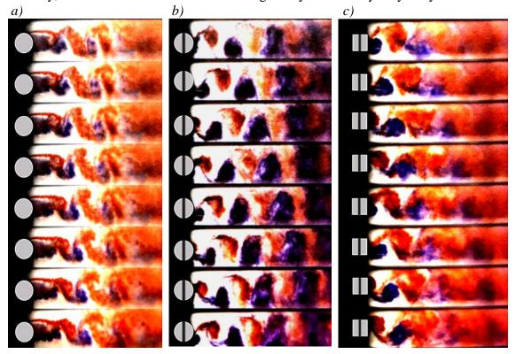
Fig. 7. Vortex generation on the bluff body:  $a - on\ a\ circular\ cylinder$ ,  $b - on\ a\ circular\ cylinder$  with the slit,  $c - on\ a\ rectangular\ cylinder$  with the slit.
