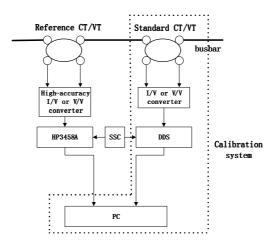
Fig.5 Block diagram of the test setup for verification of the calibration
