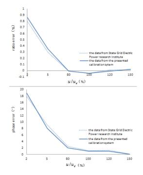
Fig.4 The normalized ratio error and phase error results of the voltage transformer comparison tests
