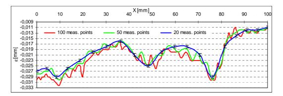
Fig. 3. Surface profiles for different numbers of measurement points
