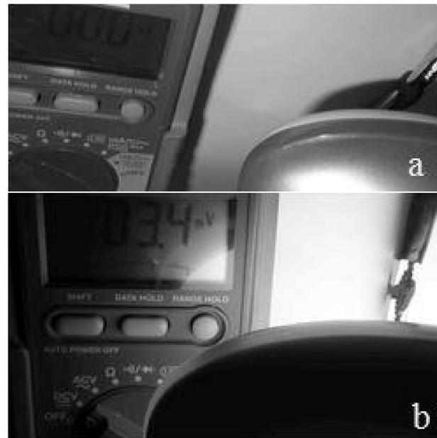
Fig. 1. Gd-paraffin sample: a) Gd-paraffin sample in an open circuit configuration held by steel electrodes; a fluorescent lamp switched of – voltage: 0 [V]; b) Gd-paraffin sample illuminated by the fluorescent lamp – voltage: 3.4 [mV].
