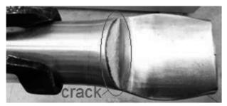
Fig. 3. Crack on the rolled oval for the roll pass 1
