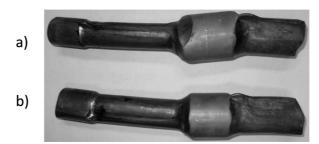
Fig. 13. Forgings from magnesium alloy AZ31 rolled in the forge rolling process: from billet with diameter  $\emptyset$  45 mm, b) from billet with diameter  $\emptyset$  42 mm
