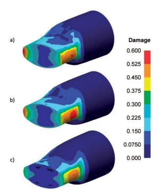
Fig. 6. Distribution of Cockroft-Latham integral value: a) segment with radius R = 10 mm, b) R = 20 mm, c) segment with gradually increasing reduction ratio
