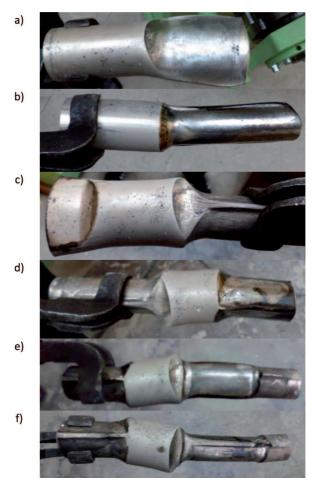
Fig. 11. Subsequent roll passes during rolling of the preform from bilet with diameter  $\emptyset$  45 mm: a) oval - I, b) circle - I, c) oval - II, d) circle - II, e) oval - III, f) circle - III
