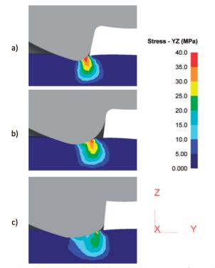
Fig. 7. Shearing stresses distribution at the moment of material clamping by segments: a) segment with radius R = 10 mm, b) R = 20 mm, c) optimized segment
