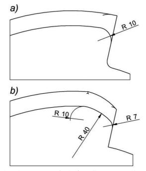
Fig. 5. Tools entrance area for the first roll pass: a) R = 10 mm, b) segment with gradually increasing reduction ratio
