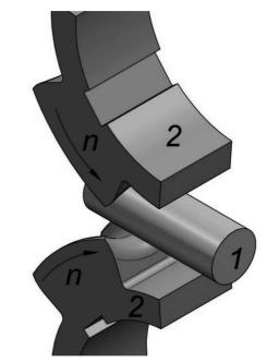
Fig. 2. Geometrical model of the forge rolling process: 1 – billet, 2 – rolling segments
