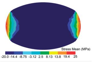
Fig. 9. Mean stresses distribution during rolling in the oval impression for the first roll pass
