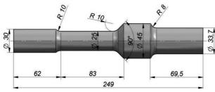
Fig. 1. Shape and dimensions of the lever preform [9]
