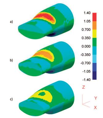
Fig. 8. Non-dilatational strains  $\gamma_{yz}$  distribution: a) segment with radius R = 10 mm, b) R = 20 mm, c) optimized segment
