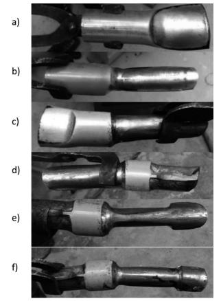
Fig. 12. Subsequent roll passes during rolling of the preform from billet with diameter  $\emptyset$  42 mm: a) oval - I, b) circle - I, c) oval - II, d) circle - II, e) oval - III, f) circle - III
