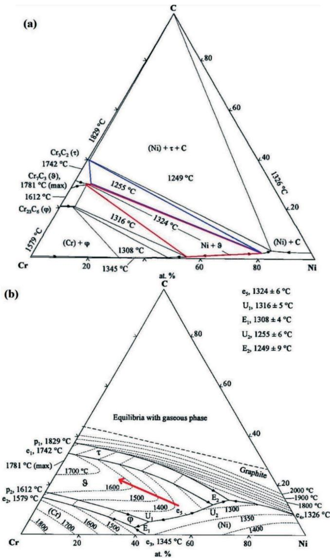
Fig. 1. Solidus (a) and liquidus (b) projection of Ni-Cr-C ternary diagram [14]
