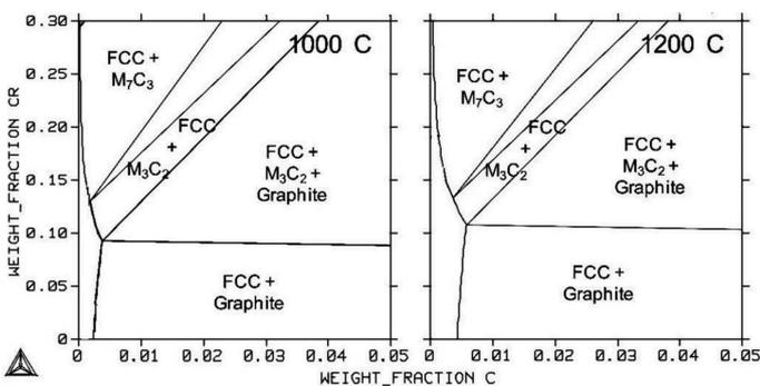
Fig. 2. Pseudo-binary isothermal cross-sections of Ni-Cr-C ternary diagram
