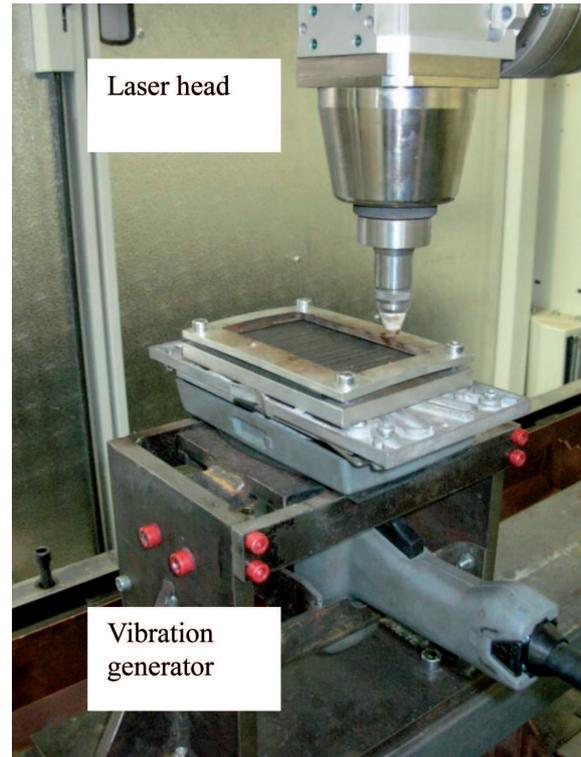
Fig. 1. Vibration-laser stand for melting metal elements
