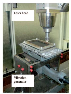
Fig. 1. Vibration-laser stand for melting metal elements
