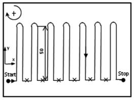
Fig. 2. Diagram showing vibration-laser melting of samples
