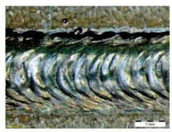
Fig. 11. Front of interfusion No. B4
