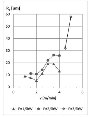
Fig. 16. Dependence of measured average roughness as a function of laser power (P) and scanning velocity  $\left(v\right)$
