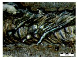
Fig. 13. Front of interfusion No. C1
