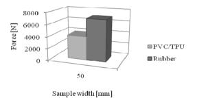
Fig. 7. Tensile strength of PVC/TPU and rubber for oil boom on 50 mm width sample
