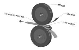
Fig. 8. Hot wedge or hot air welding [9]
