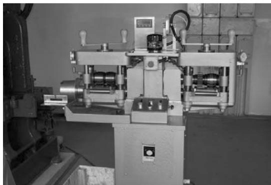
Fig. 1. Stand for repetitive corrugation and straightening of strips
