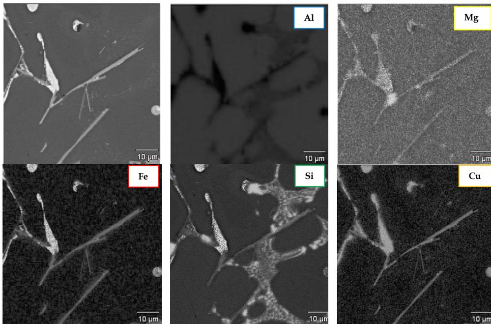
Fig. 3. SEM image of the C355.0 alloy and corresponding elemental maps of: Al, Mg, Fe, Si and Cu
