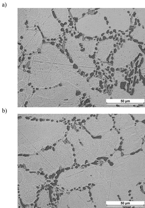
Fig. 6. The microstructure of C355.0 alloy in the T6 condition (a,b)
