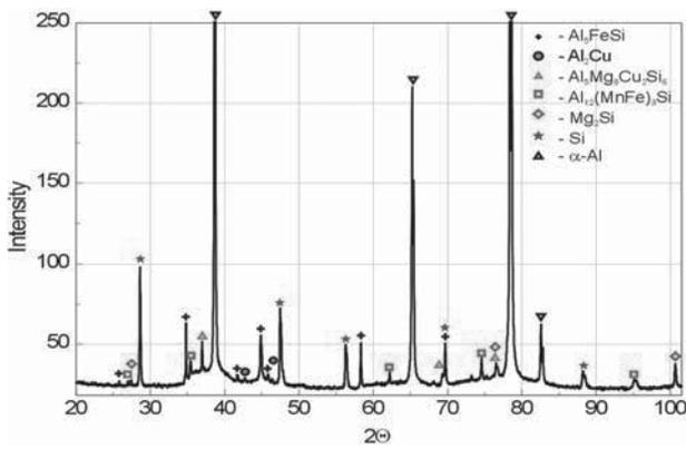
Fig. 5. X-diffraction pattern of C355.0 alloy in as-cast state
