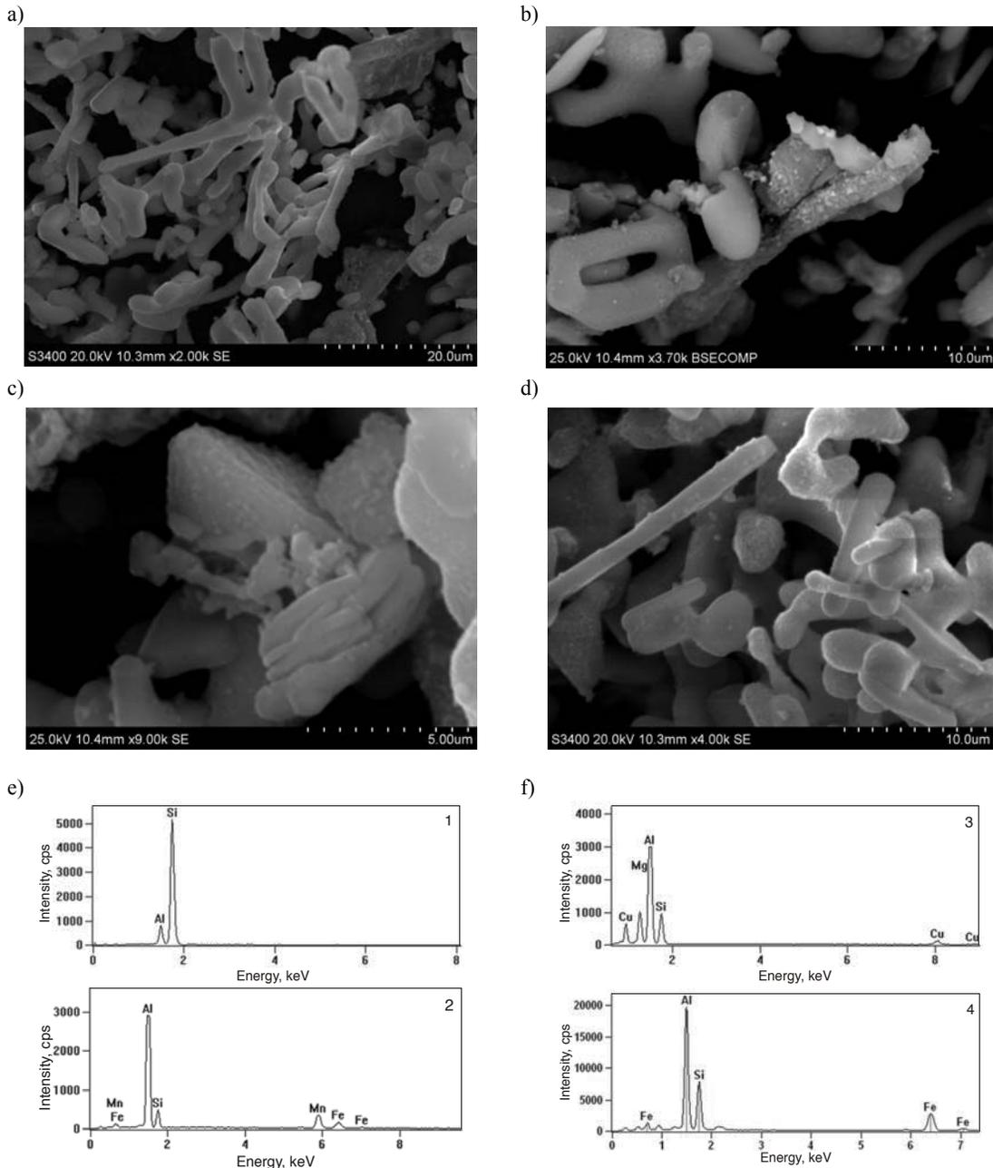
Fig. 8. SEM micrographs (a-d) of the particles extracted from the C355.0 alloy and EDS spectra (e,f)
