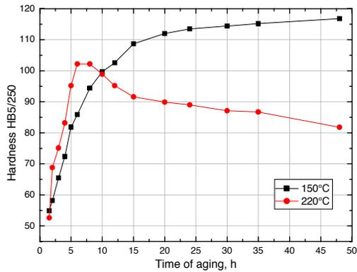
Fig. 9. Variation of hardness with time of aging of investigated alloy at temperature of 150 and 220°C
