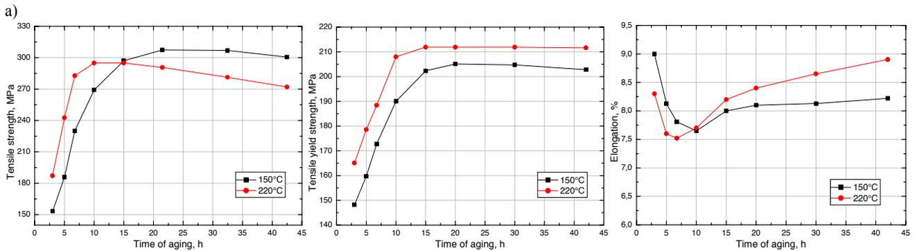
Fig. 10. Effect of aging time on: a) tensile strength, b) tensile yield strength and c) elongation of C355.0 aluminium alloy aged at 150°C and 220°C
