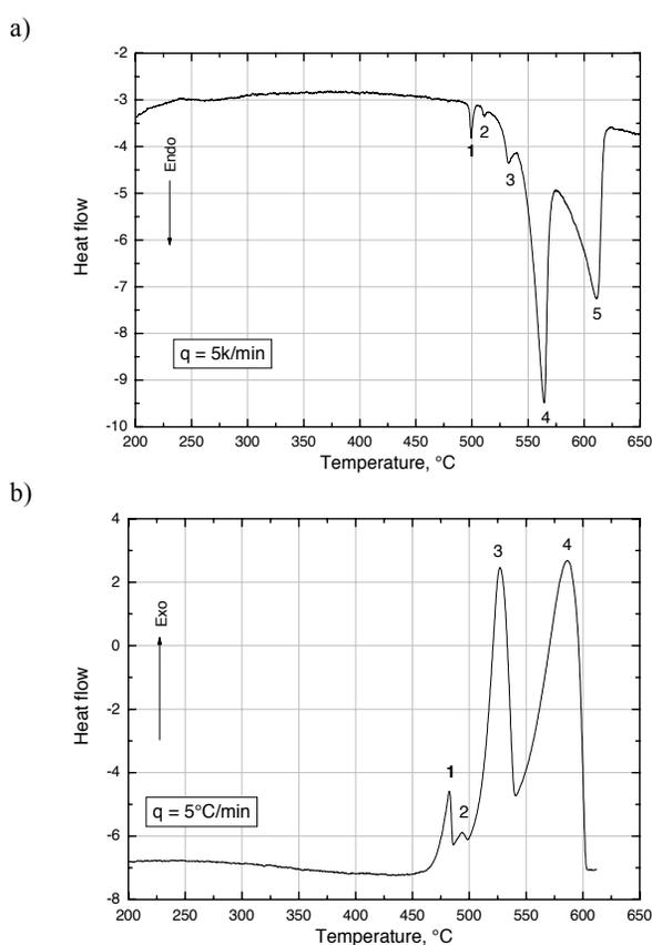
Fig. 1. DSC thermograms of as-cast specimens of C355.0 alloy, obtained during a) heating and b) cooling at rate of 5°C
