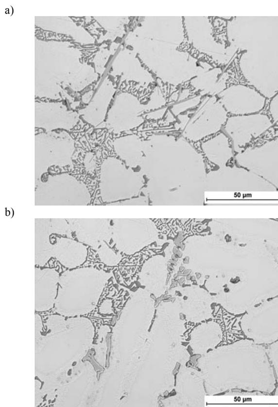
Fig. 2. Morphology of C355.0 alloy in the as-cast state: (a) unetched and (b) etched.
