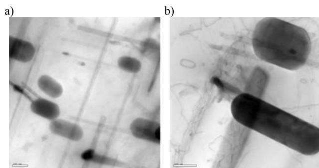
Fig. 12. Precipitation of strengthening  $\beta$ -Mg<sub>2</sub>Si i  $\theta'$ -Al<sub>2</sub>Cu phases in C355.0 (a,b) - TEM
