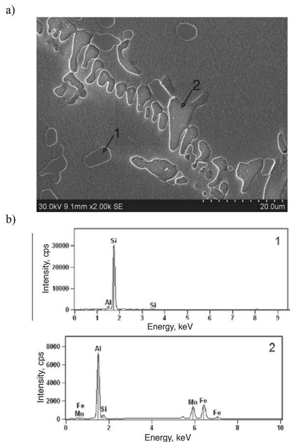
Fig. 7. a) SEM micrographs of the C355.0 alloy in the T6 condition; b) the corresponding EDS-spectra acquired in the positions indicated by the number 1 and 2.
