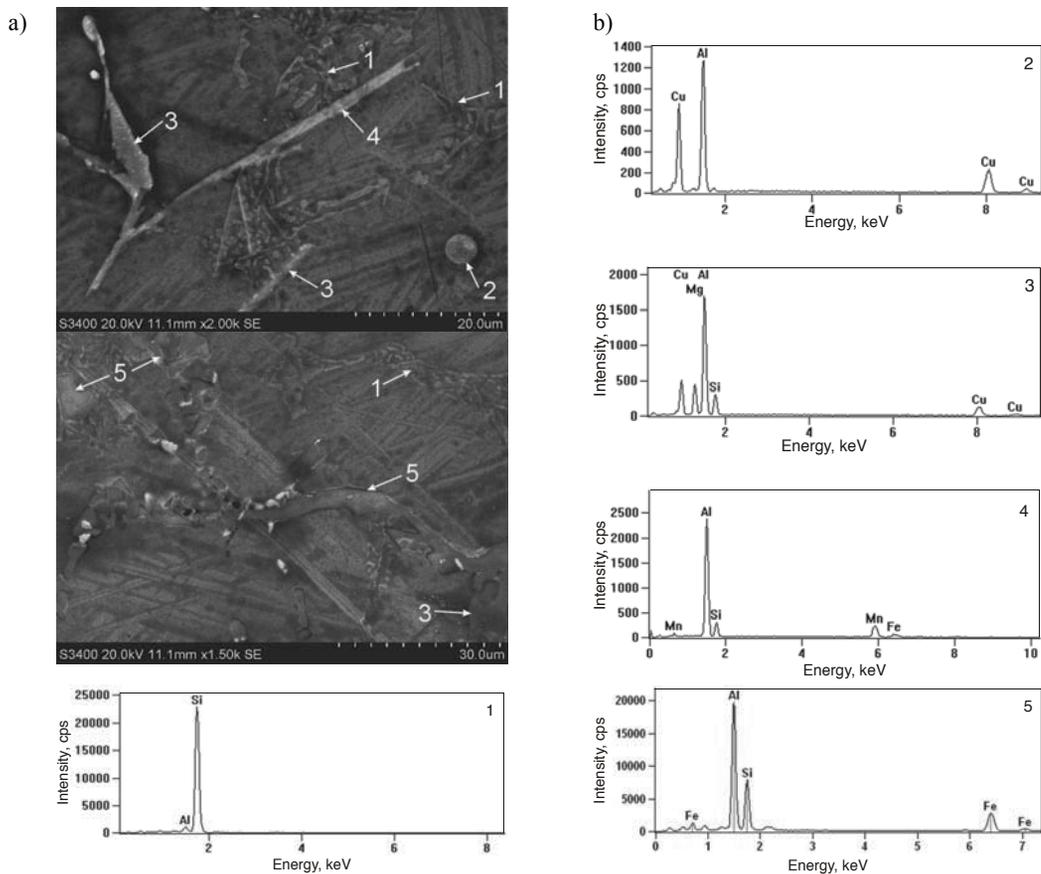
Fig.4. a) SEM micrographs of the C355.0 alloy in the as-cast state; b) the corresponding EDS-spectra acquired in positions indicated by the number 1 and 2.
