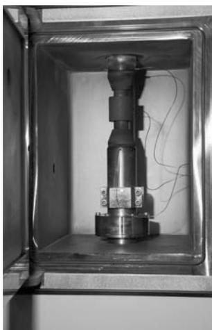
Fig. 2. Graphite die with ceramic powder before sintering process
