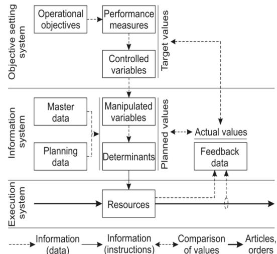
Fig. 2. Elements of the operational logistic action system [6].
