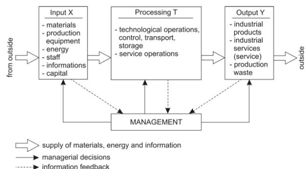
Fig. 1. Production system model (according to [4]).
