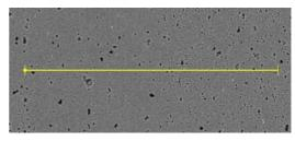
Fig. 14. Fragment of the structure from Fig. 8. Welding parameters:  $\omega = 900 \text{ min}^{-1}$ , V = 224 mm/min. Triflute pin. SEM-EDS chemical composition analysis was conducted along the marked line (Fig. 15)
