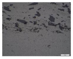
Fig. 11. Fragment of the structure from Fig. 6. Joining of EN AC-43200 metal layer (from top) with EN AW-6082 alloy
