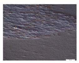
Fig. 10. Fragment of a structure from Fig. 6. EN AC-43200 alloy (from top) located on the advancing side after friction welding process (Nomarski contrast)
