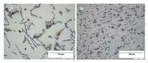
Fig. 18. Structures of casting alloy before FSW – a) and after FSW process – b) (SEM)
